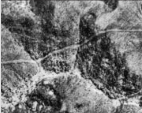
Figure 1. Aerial image prior to rectification. Note the displacement of a utility right-of-way due to topographic relief.
